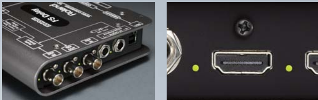
Connectors fastened with nuts or screws. LED input indicators for confirming signals
