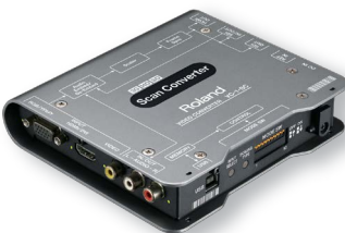
Scan Converter VC-1-SC Conversion of digital signals of SDI and HDMI and analog signals of RGB, component and composite to SDI or HDMI
