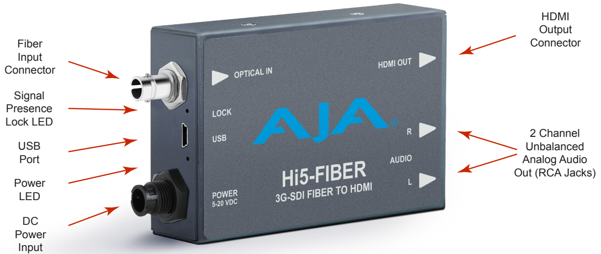
Figure 2. Hi5-Fiber Converter Connections
