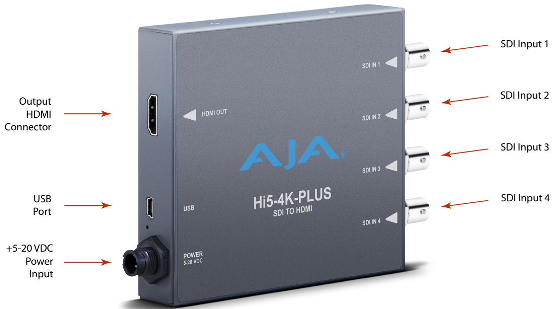
Figure 2. Hi5-4K-Plus Converter Connections
