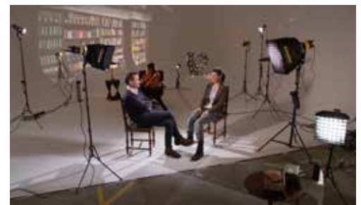
Picture above shows increased depth illusion, enhanced by placing background (book shelf projection) out of focus.
